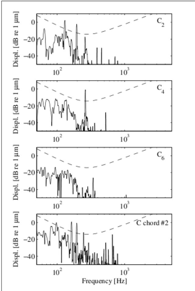
**Figure 3.** Spectra of the tactile response of a Bösendorfer grand piano measured at the keyboard (solid line), along with perceptual thresholds for the palm from Verrillo [12] (dashed line). Examples given for notes  $C_2$ ,  $C_4$ ,  $C_6$ , and the  $C$  chord #2, all played at *forte* level.
