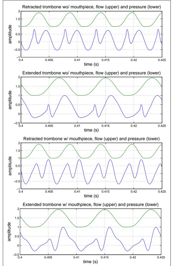
**Figure 6.** Synthesis examples using parameter values from Table 1 and Table 2, showing flow versus bell output pressure (produced sound) in a note's steady state, with slide in both retracted and extended positions, and with and without a mouthpiece.
