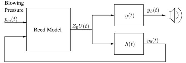
**Figure 2.** A convolutional synthesis approach to the signal flow diagram shown in Figure 1, with signals  $h(t)$  and  $g(t)$  being the impulse responses of the instrument tapped at the positions  $y_0(t)$  and  $y_L(t)$ , the inverse transforms of (1) and (2), respectively. The input pressure is the product of the characteristic (wave) impedance  $Z_0$  at the mouthpiece and the volume flow  $U(t)$ , a signal generated by a reed model in response to a blowing pressure  $p_m(t)$ .
