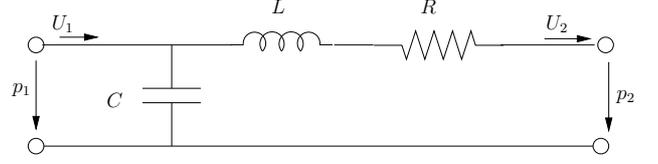
**Figure 5.** The system diagram for the mouthpiece model. The cup volume is represented by the capacitor, and the attached narrow constriction is modeled as a series inductance  $L$  and dissipative element  $R$ , which accounting for wall losses.
