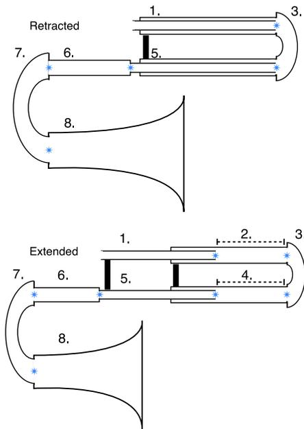
**Figure 3.** Interior view of trombone, in both fully retracted and fully extended positions, showing assembly of components from Table 1.
