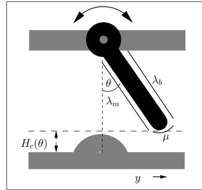
**Figure 4.** The blown open configuration of the generalized valve model, showing geometric parameters  $\lambda_m$ , the length of the valve that sees the mouth pressure,  $\lambda_d$ , the length of the valve that sees the valve’s downstream pressure, and  $\mu$ , the length of the valve that sees the flow. Changing these parameters will change the corresponding component forces of the overall driving force  $F = F_m + F_b + F_U$ .
