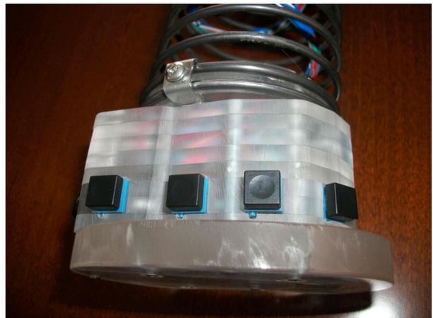
Figure 3. Left hand controller, 4 push buttons displayed
