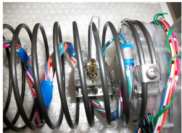
**Figure 7.** Measuring length variation with a joystick
