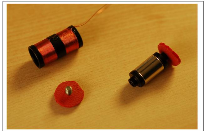
**Figure 3.** One of the actuators as used in [15] (Photo by courtesy of J. Malloch).
