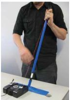
Figure 7 Gametrak Chordophone An analysis of attack events (based on impulses on the x- and y-axes) determines whether the musician has plucked a string and to what extent the string deviated from its average position.
