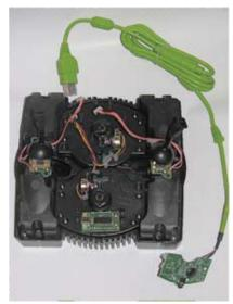
Figure 10: replacing the microcontroller
