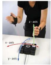
Figure 2: Tethered Theremin control axes
