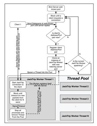
Figure 1. Multi-client concurrent server algorithm
