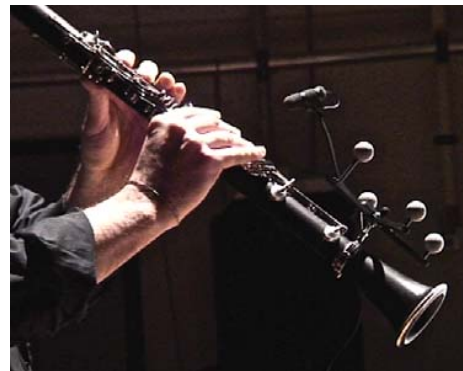
Figure 1. A 4-marker tracking target mounted on a clarinet using a Marschgabel fitting (and microphone attached)
