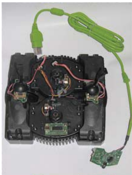
Figure 10: replacing the microcontroller
