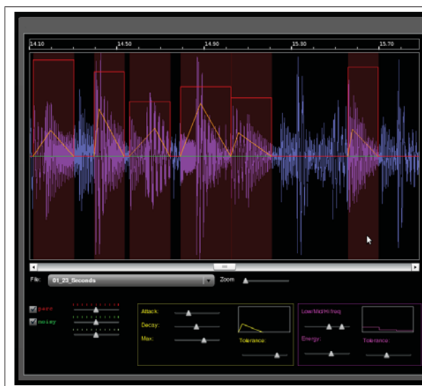
Figure 3. Interface of the exploration prototype. Three sound objects are identified. Amplitude envelope for the percussive objects (red) are represented with triangles.
