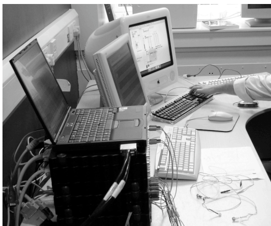
Figure 5. The demonstration system runs on two computers. The laptop performs the EEG analysis with Matlab/Simulink and the Macintosh generates the music with Max/MSP and Common Lisp. The units under the laptop are the EEG amplifiers.
