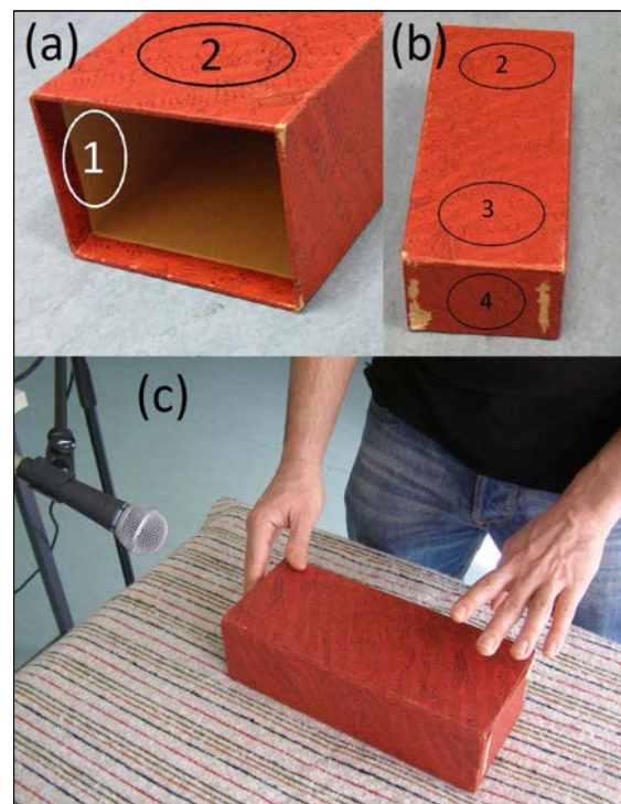
Figure 1. A box made of recycled paper. Impact regions 1 and 2 are shown in (a) while regions 2, 3 and 4 are shown in (b). The placement of the microphone with respect to the object and the general setting for playing the object is shown in (c).
