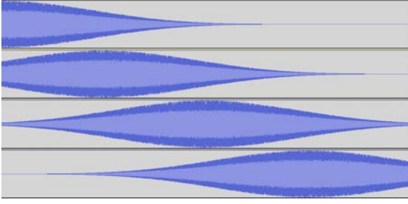
Figure 5. Signals of four speakers of a sound source turning around the listener. In-phase decoding 4th order.
