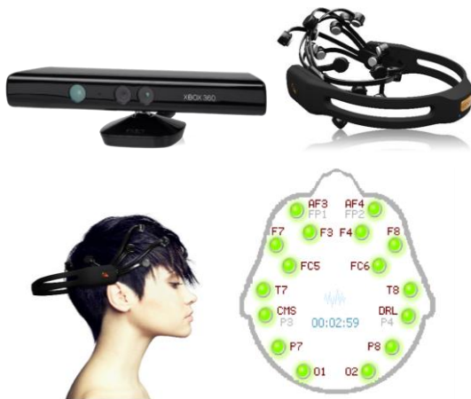
Figure 2. The technological mediators used in “Brainswarm” to capture the bio-conductor’s body/hand gestures (MS Kinect-top left) and EEG brain activity via the EEG Emotiv interface (top-right). The way the latter is used and the corresponding recording sites on the brain are shown in bottom-left and bottom-right, respectively.
