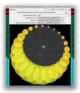
Figure 5: Push transform plugin interface.
