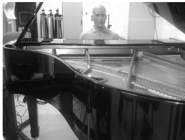
Figure 1: Setup for loudness estimation on the grand piano (PD) using a KEMAR mannequin.
