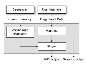
Figure 10 Voicing algorithm global structure
