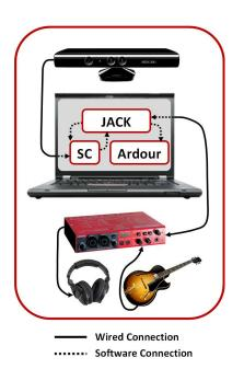
Figure 3. Configuration of the system's hardware and software components.
