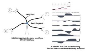
Figure 3. The robot orients its tool at different configurations to approach the same point and the change in joint angles of the 6DOF arm is shown on the right.
