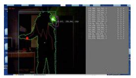
Figure 2. Blob analysis of the human body and the hand in separate planes. The red curve is the robot path inside the human body contour.
