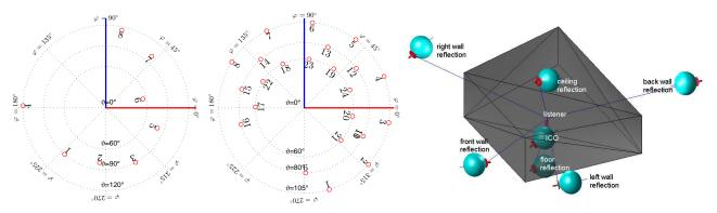
**Figure 2**. Layouts of the pieces *grrawe* (left) and *firniss* (middle) in terms of beams (see numbers) to which the composition routes and amplitude-pans its signal objects. The image on the right shows the mirror sources representing wall reflections of the ICO, cf. Tab. 1, including an examplary beam pattern pointing at the back-wall reflection.
