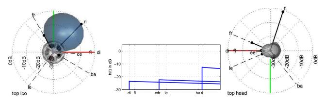
**Figure 4**. Reflection paths as they are excited by the stimulus example *squeaks* through the ICO are shown in the polar top view (left). Time sequence of arriving reflections at the listener and their *echo thresholds* are shown in the middle. The polar top view on the listener (right) shows from where reflections arrive with which propagation decay.
