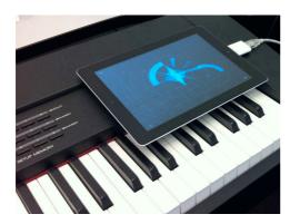
**Figure 4**. TC-Data running on an iPad, connected to an external MIDI interface. The MIDI controller data can be merged with the keyboard output.
