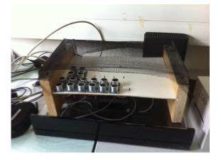
Figure 3. Ultrasound matrix, for eight keys.
