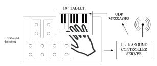
Figure 4. Augmented reality system schema with ultrasonic hit detection.
