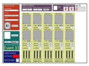
**Figure 9.** The part of the MAX/MSP 6.1 interface that monitors the biosensors' status and swarms' parameters, along with the elapsed time and the CPU overloading.
