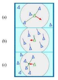
**Figure 4**. The three main cahracterstics of a swarm boid behavior with its flockmates: (a) separation, (b) alignment, and (c) cohesion.
