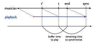
**Figure 5**: The diagram represents the different values to be considered for the speed calculation. At the current time t, the dates end (the canon end) and sync (the final synchronization point) are estimated according to the tempo value. The  $t^\prime$  value corresponds to the time at which the live musician played the current position of the buffer.
