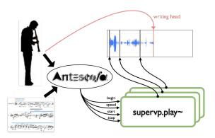
**Figure 3**: *Antescofo* follows the clarinetist's performance which is recorded in parallel into a buffer. Phase Vocoder objects read this buffer at specific positions and speeds controlled by *Antescofo* as outlined in the score.
