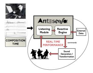
**Figure 2**: General architecture of Antescofo. The score is an input of both the listening machine and the reactive engine. The events recognized by the listening machine are signaled to the reactive engine which schedule the actions at the right time.
