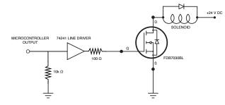
**Figure 9**. Kritaanjli's solenoid circuit. A line driver is used to allow for longer cable runs between the microcontroller and the Persephone board. The same circuit is used for Kritaanjli's bellows pumping motor.
