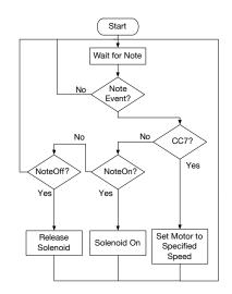
Figure 8. The program flow of Kritaanjli's firmware.
