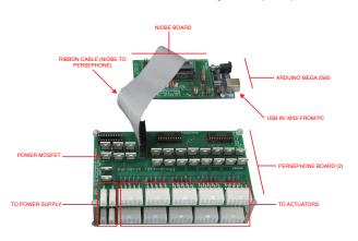
**Figure 7**. Kritaanjli's electronics: an Arduino is connected to two 24-output Persephone boards by a Niobe board.
