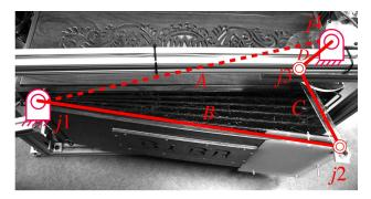
**Figure 5**. Kritaanjli's four-bar linkage bellows-pumping mechanism. The crank is visible on the image's right; the rocker (the hinged harmonium bellows) is on the image's left. Overlaid on the image is a drawing of the assembly's elements.
