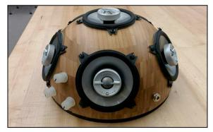
Figure 5b. 6-channel hemispherical speaker
