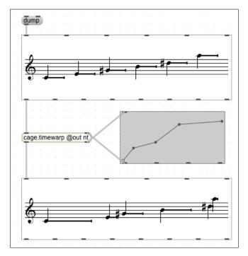
**Figure 4**. An example of temporal distortion performed through cage.timewarp. The function in the  $lambda\ loop$  associates time in the original score (above), represented on the x-axis, to time in the resulting score (below), represented on the y-axis.
