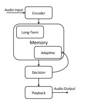
Figure 3: System diagram for Flight computational agent.
