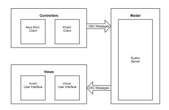
Figure 5. The Kuatro MVC Architecture.
